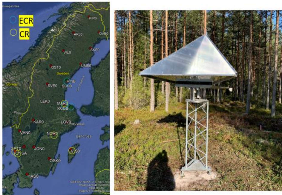
Figure 4: Left: The approximate locations of the electronic corner reflectors (ECR) and passive reflectors (CR) which are co-located with permanent GNSS stations (solid red circles). Right: Trihedral triangular passive corner reflector installed in Mårtsbo.
